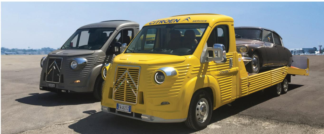
The New Type H can be the condign transport vehicle for your classic car, equipped with lightweight fixed platform, hydraulic telescopic back fork or low frame and fixed platform, suited for supercars as well.
